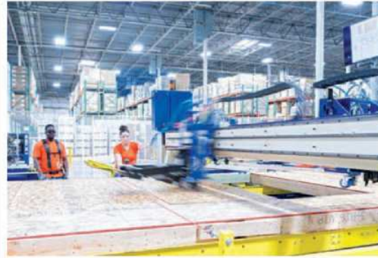
At a factory in Phoenix, Katerra staffers and robots build prefab wall panels on an assembly line
